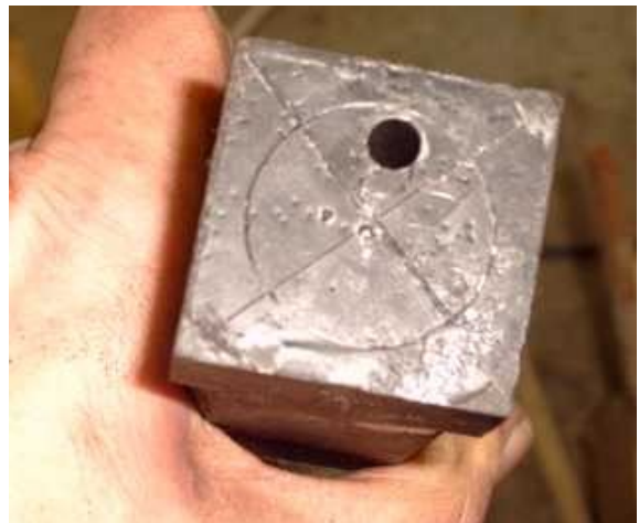
Illustration 6: The middle bore, seen from the headstock end after boring, showing some drift
