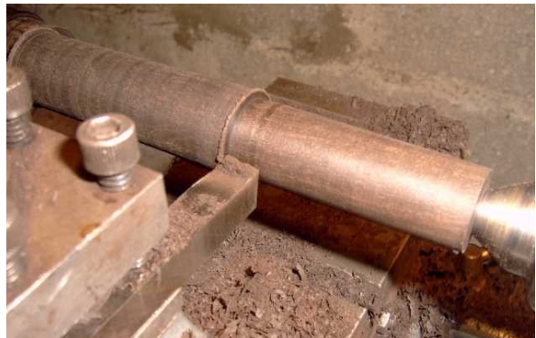
Illustration 9: Turning down the slide tenon before final boring
