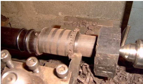
Illustration 7: Turning the reed tenon
