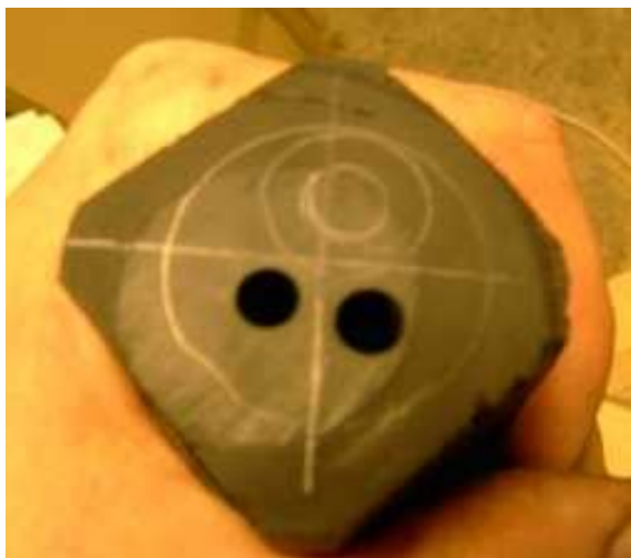
Illustration 8: Slide tenon end plan
