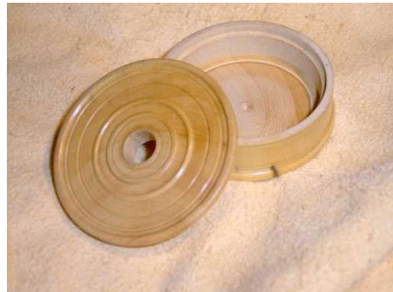
Illustration 13: The completed boxwood puck ready for gluing
